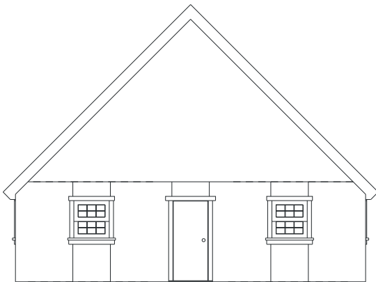
Figure 6.12: The elevation after a hidden line removal
