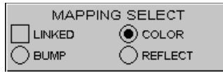
Figure 45. The Mapping Select options determine which image map is being manipulated in the Object Designer viewport.
