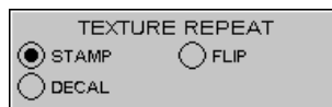
Figure 47. The Texture Repeat options determine how a texture is repeated as it is mapped onto an object.
