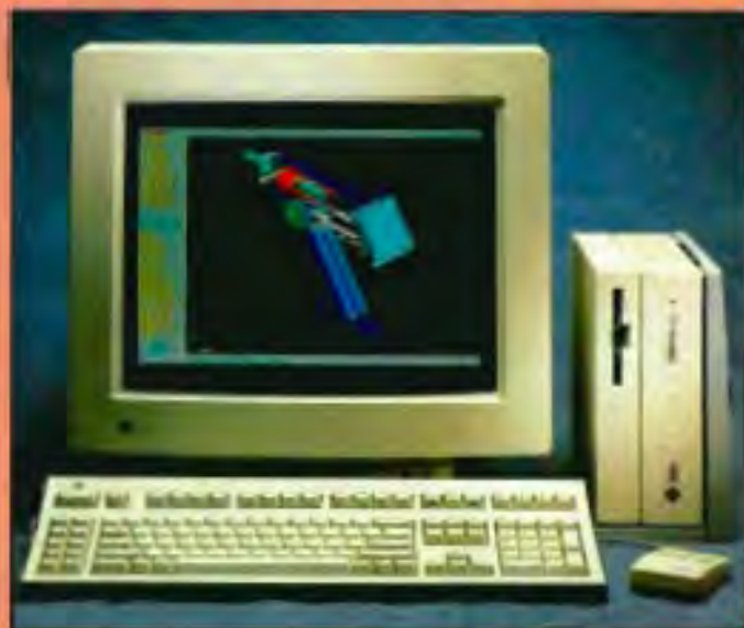
The SPARCstation™ LX is the industry's least expensive graphics workstation, shown here running CADKEY software. The new system features the GXplus accelerator, CD-quality audio and built-in ISDN (Integrated Services Digital Network).
