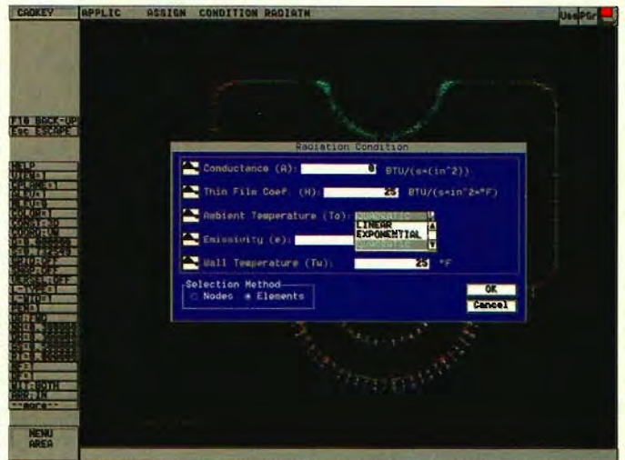
The dialogue box above is used in assigning the thermal radiation boundary condition. A distribution function is being applied to set the ambient temperature parameter.
