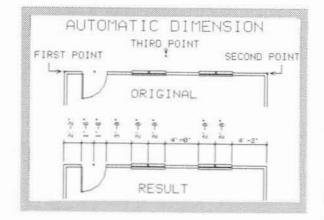
The Automatic Dimensioning command of the new DataCAD 3.0.
