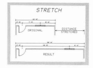
The DataCAD 3.0 Associative Dimensioning command used in combination with the Stretch command.
