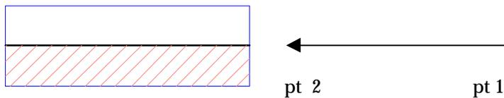
If you need to change the orientation of the wall definition after you complete your drawing, press [Alt] + [F] to go to the CleanUp menu, choose DefOuter, and click on the outer side of the wall. DataCAD Plus reorients the wall definition.
