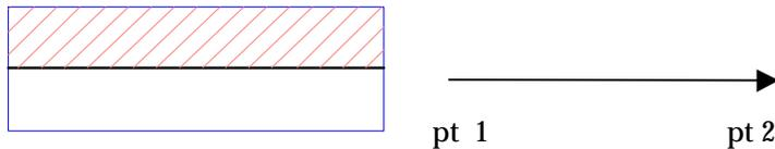
Drawing the wall in a counter-clockwise direction will result in this display:
