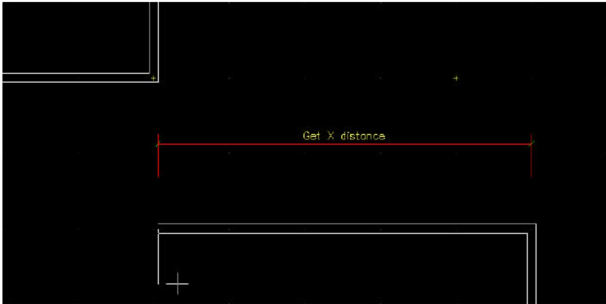
Figure 4: The horizontal wall is drawn, based on the distance between the vertical wall end and the building corner you selected using Get-Snap.
