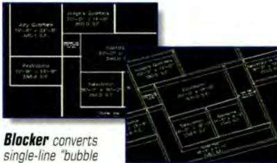
**Blocker** converts single-line "bubble diagrams" to walls instantly, then auto-calculates square footage and room dimensions.
